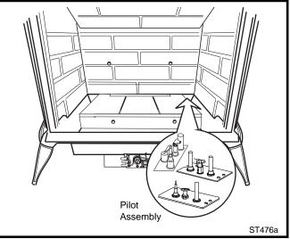
Fig. 48 Pilot Assembly location.
